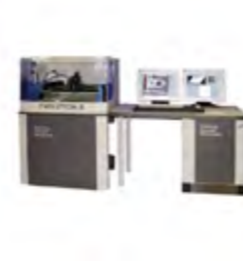
Scanning Acoustic Microscope (SAM) Evolution II transducers: 20 MHz, 30 MHz, 50 MHz, 75 MHz, 110 MHz
