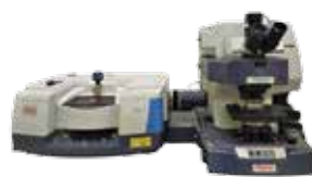
Nicolet iS50 Fourier Transform Infrared Spectrometer (FTIR) Spectral Range: 350-7800 1/cm-1
