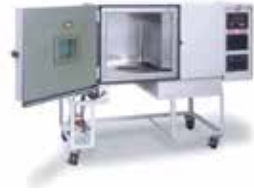
High or Low Temperature Storage Test Chamber Tenney BTC: -73°C to 200°C Enviro Oven M0384: 30°C to 300 °C
