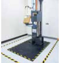
Drop Test ISO 2248-1985, GB/ 148575-92, JIS Z0202-1994 Maximum Drop Height: 1.5m Maximum Load Weight: 80kg
