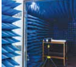
Semi Anechoic Chamber Conducted Emission and Radiated Emission 150 kHz to 2.5 GHz
